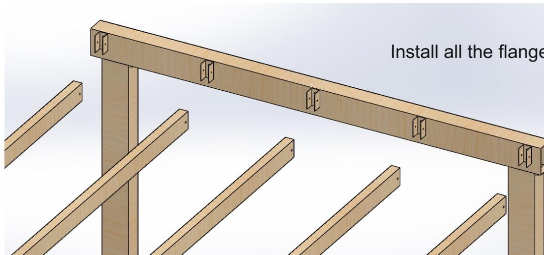
Install all the flanges to the front carrier profile
