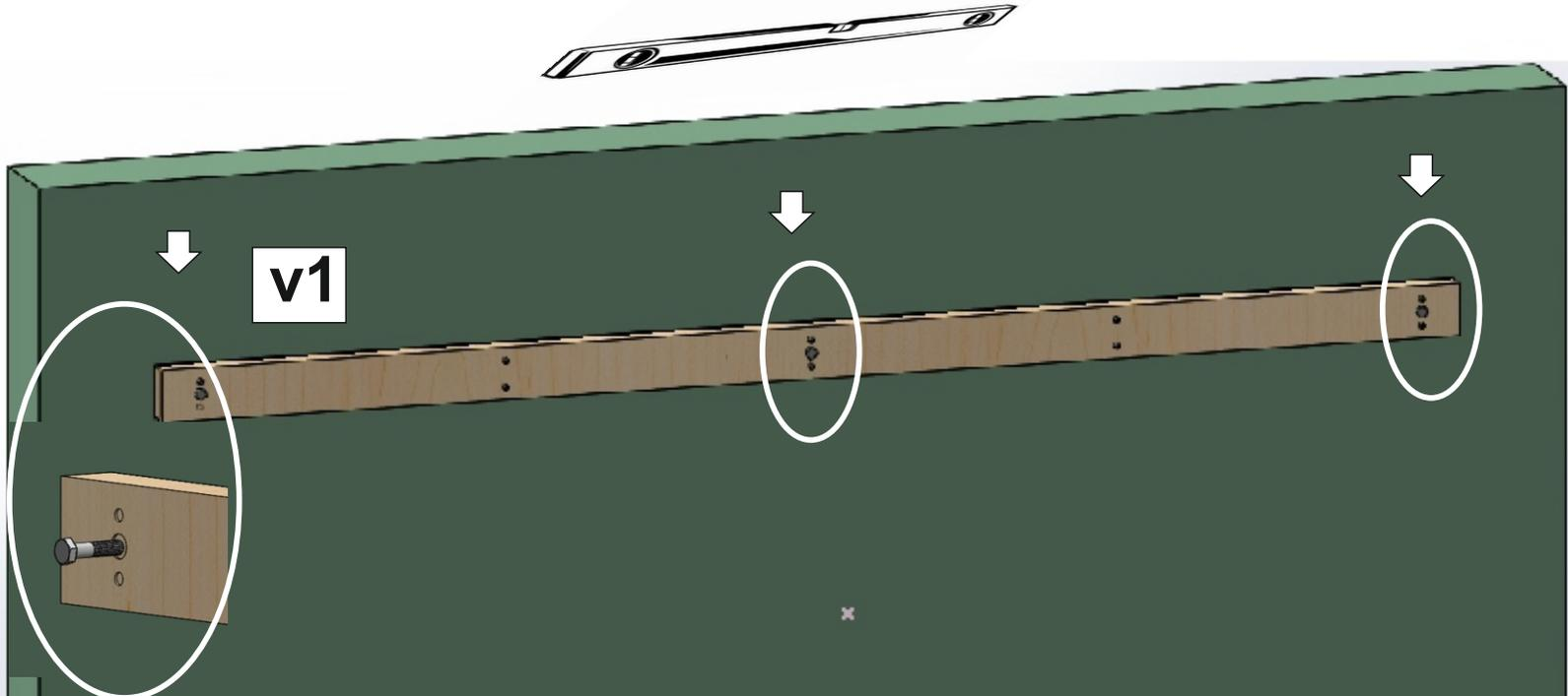
Screw the flange to the wall support profile with the screw V5
