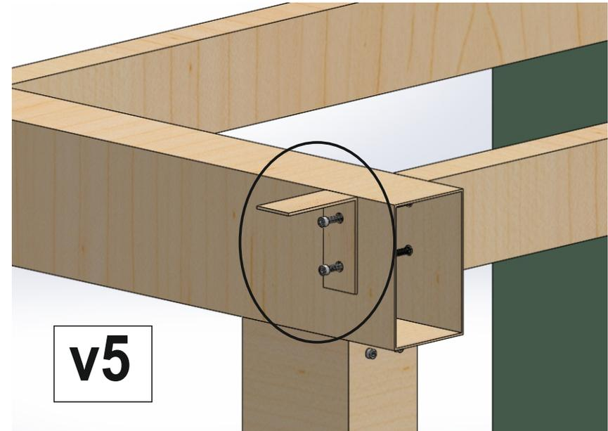
Place and install the front angle profile with V5
