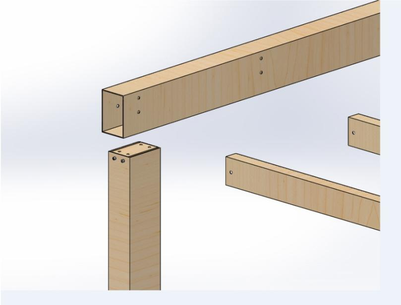
Screw the front carrier profile to the post profile with the screw V5
