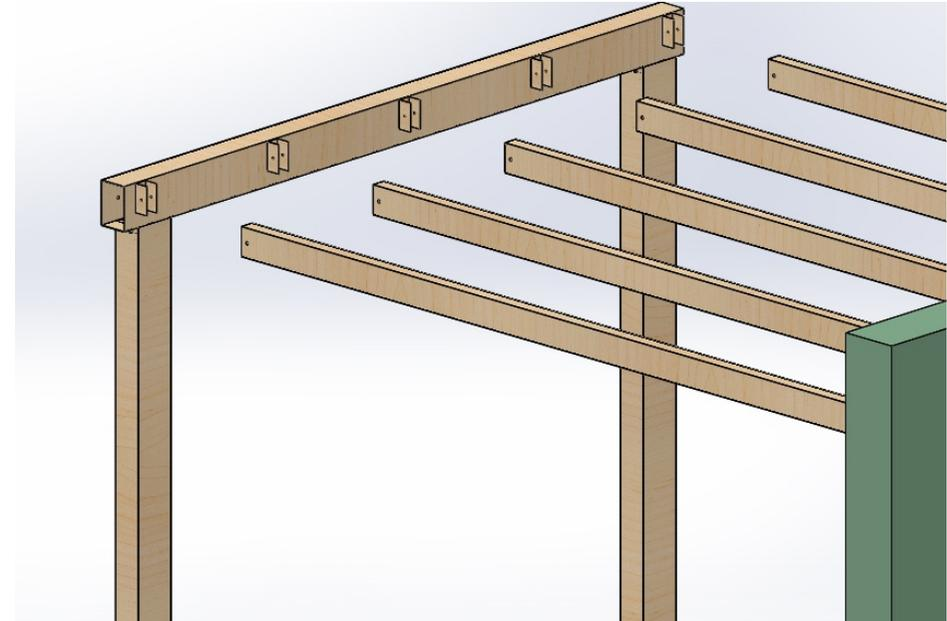
Screw to front carrier profile the flage with the screw V5
