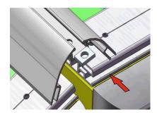
Slide the nut on the gap to profile
