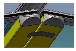
Place the rain cover profile holder between the profiles from bottom side
