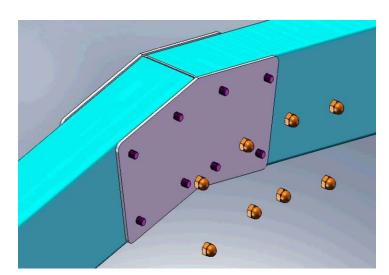
Place the screws to the holes and tighten the nut form both side
