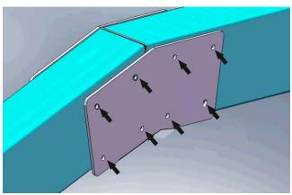
After the correct installation of carports, place the upper stabilization plate and drill with a drill bit of 9 mm from both side.
