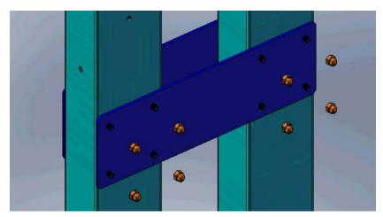
Place the screws to the holes and tighten the nut form both side
