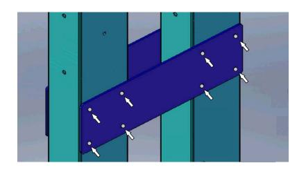
After the correct installation of carports, place the side stabilization plate and drill with a drill bit of 9 mm from both side.
