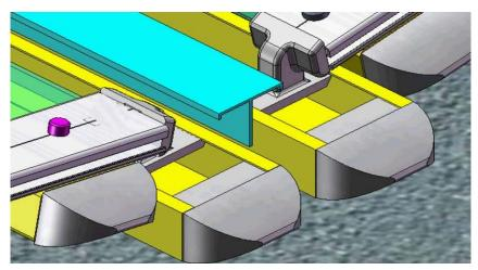
Place the T profile between the rain gutter
